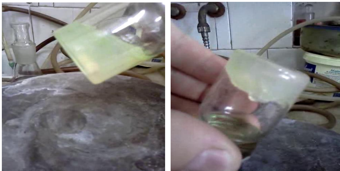
Figure 1. Photographs of gel-like reaction mixtures after 25 (left) and 50 (right) seconds of the reaction
